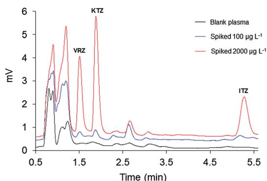
Fig. 8 Chromatograms obtained from MCM-41-SPMTE of blank azole drugs and spiked azole drugs at 100 and 2000 ppb.
