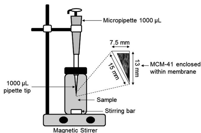
Fig. 1 Schematic representation of MCM-41-SPMTE system.
