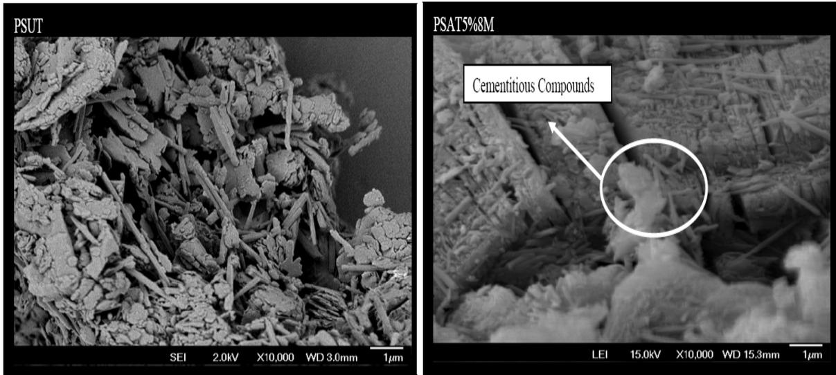
Fig. 2 FESEM images of natural (PSUT) and acid treated samples (PSAT5%8M).
