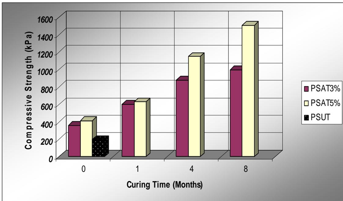
Fig. 3. Strength development for Pink Soil mix designs with curing time.
