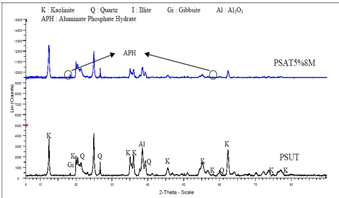
Fig. 1. XRD patterns of untreated (Bottom) and 5% phosphoric acid-treated soil (Top).
